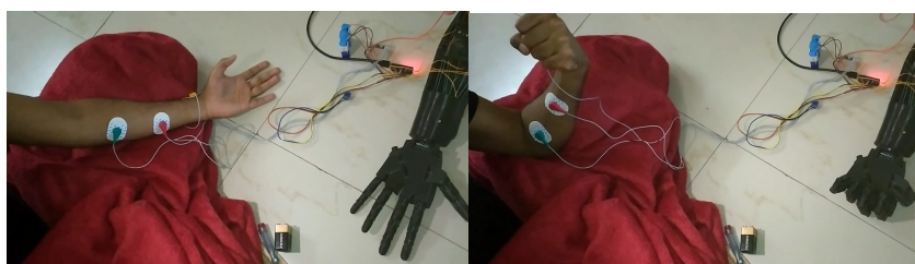
Fig. 15: opening and closing of fingers in the final prototype
