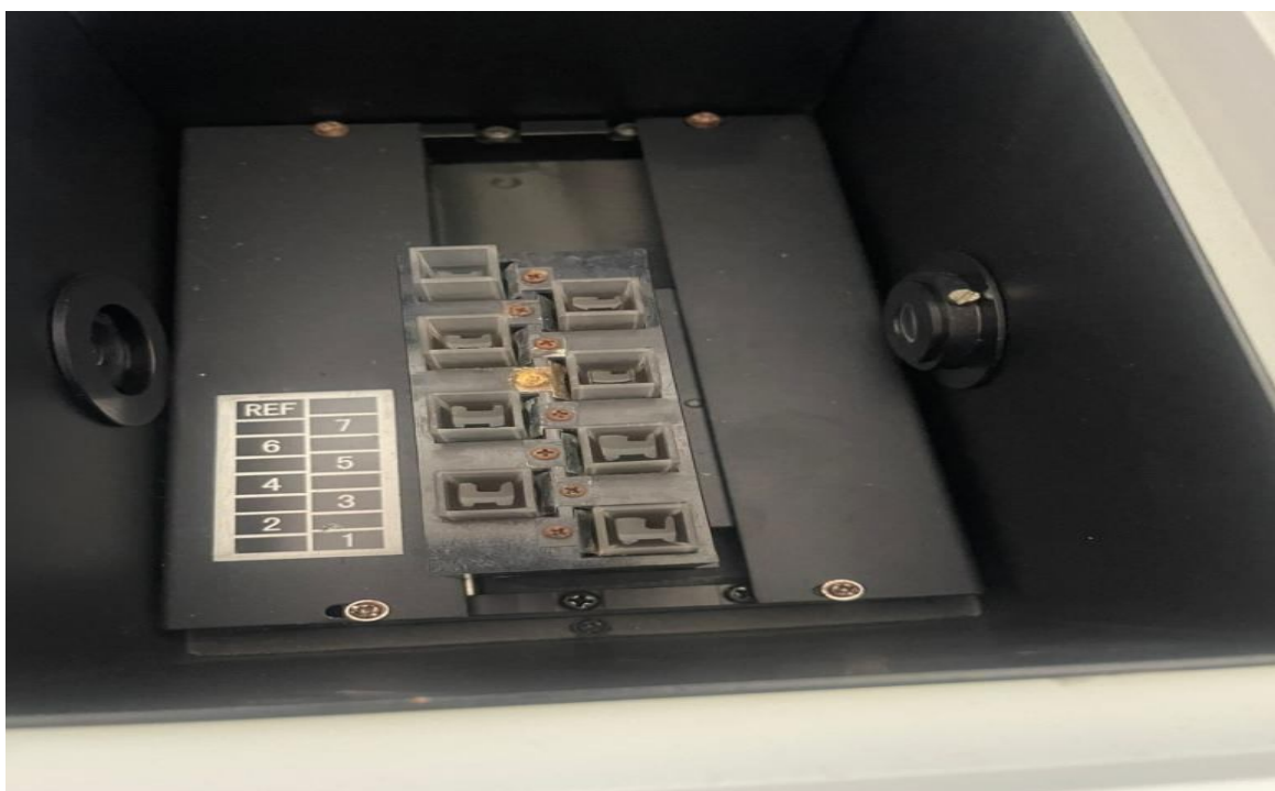
Figure 23: Samples placed in cuvette for spectroscopy
