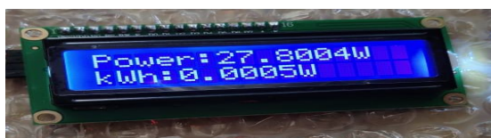
Fig-10.2 Power and kWh in LCD Display
