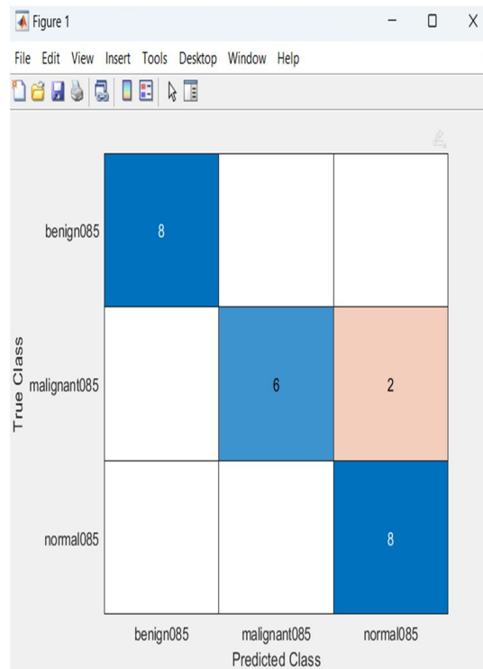
Fig. 7. Confusion Matrix for Dataset 2 Using SVM accuracy=91.66% overall precision=93.33% overall recall=91.66% f1_score=92.49%
