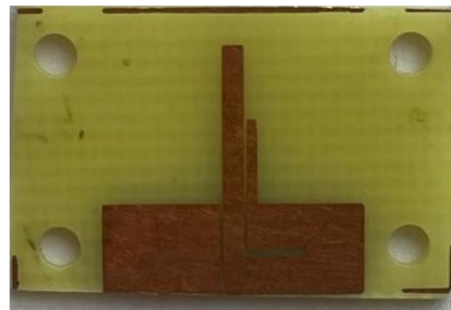
Fig. 4. Final Antenna Design Fabricated
