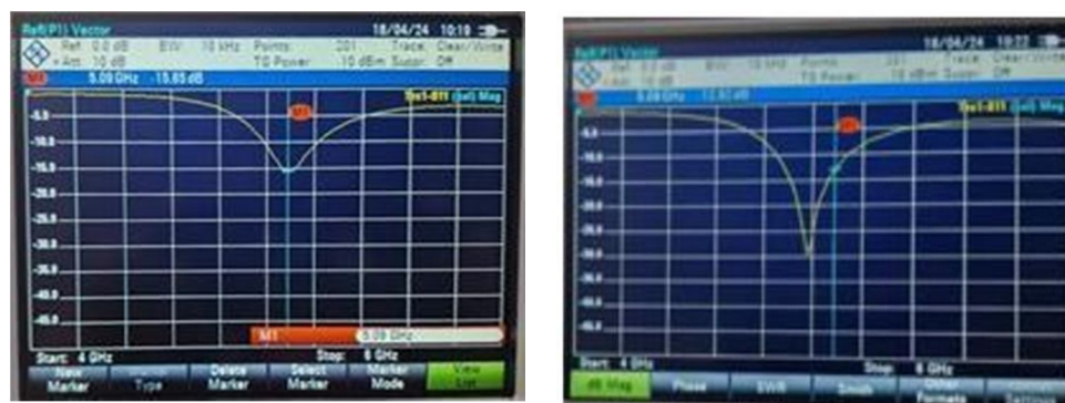
Fig. 5. S11 Results for Fabricated Final Design a) without substrate and b) with superstrate
