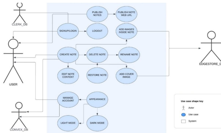
Figure 2.1 Use Case diagram
