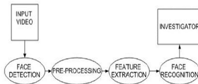
Fig. 3. CCTV Recognition Process.
