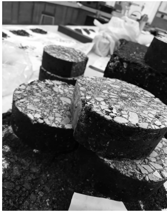
Fig. 4 NANO CLAY MODIFIED BITUMEN MOULDS
