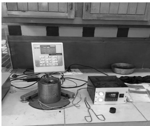
Fig. 3 EVALUATION OF VISCOSITY BY ROTATIONAL VISCOMETER
