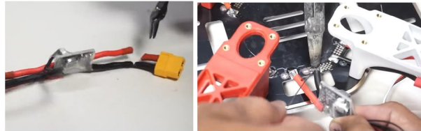
Fig 23 - Power module soldering
