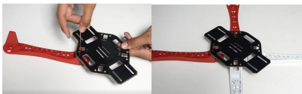
Fig 20 - Frame lower base setup
