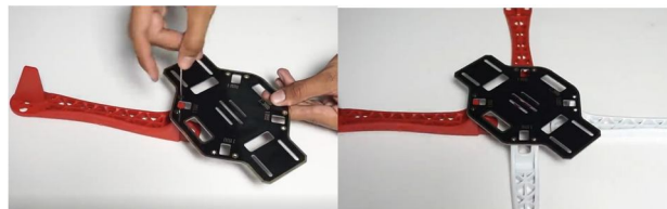
Fig 20 - Frame lower base setup
