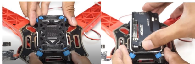
Fig 25 - Flight controller setup
