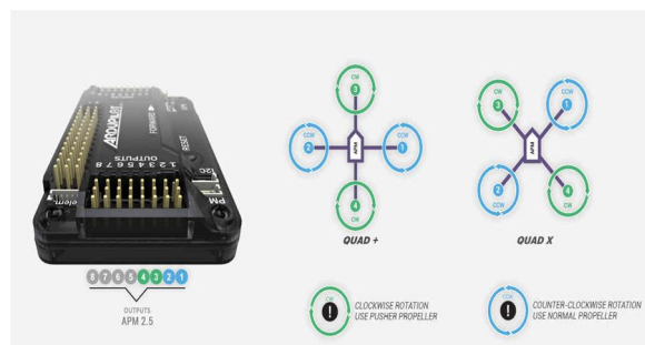
Fig 25 - Flight controller motor setup
