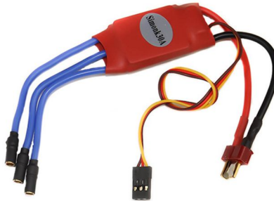
Fig 8 - ESC ( Electronic Speed Controller)
