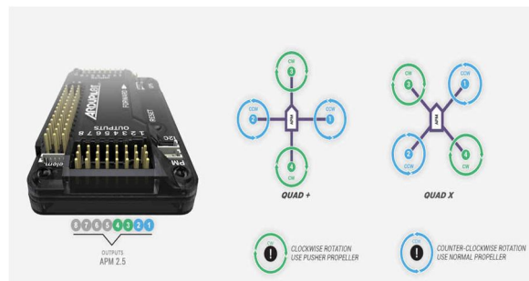
Fig 25 - Flight controller motor setup
