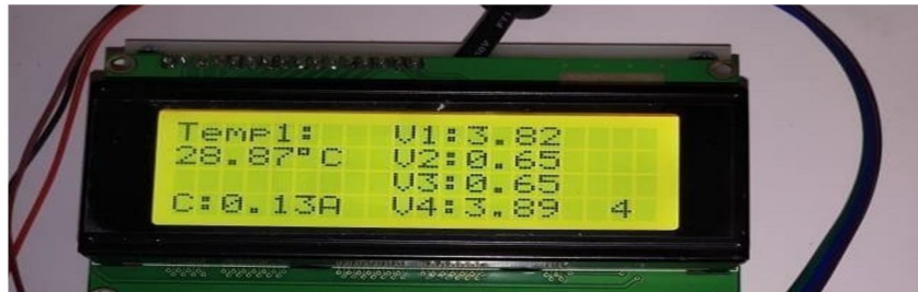
Figure 15: LCD display showing performance parameter
