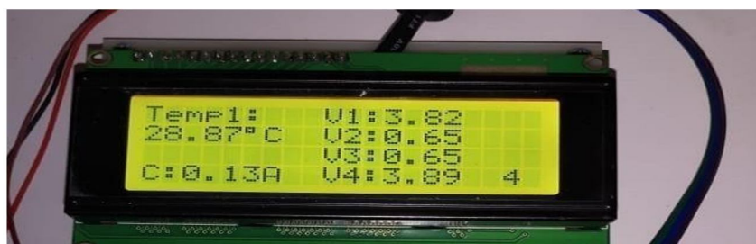
Figure 15: LCD display showing performance parameter
