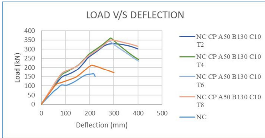
Fig 4 h: Load v/s deflection curve NC CP A50 B130 C10 with varying thickness
