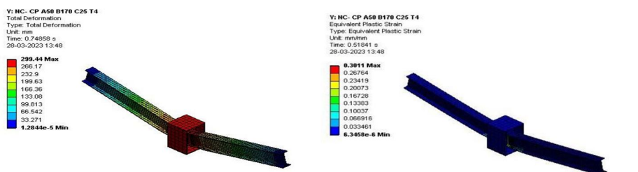
Fig 5 c: Total deformation and equivalent plastic strain of NC CP A50 B170 C25 T4
