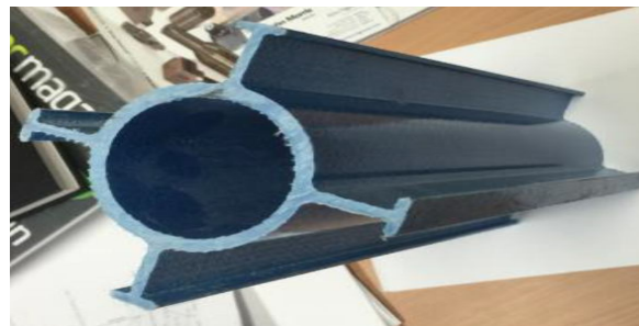
Fig. 1 Hollow Composite Reinforced Section (HCRS)
