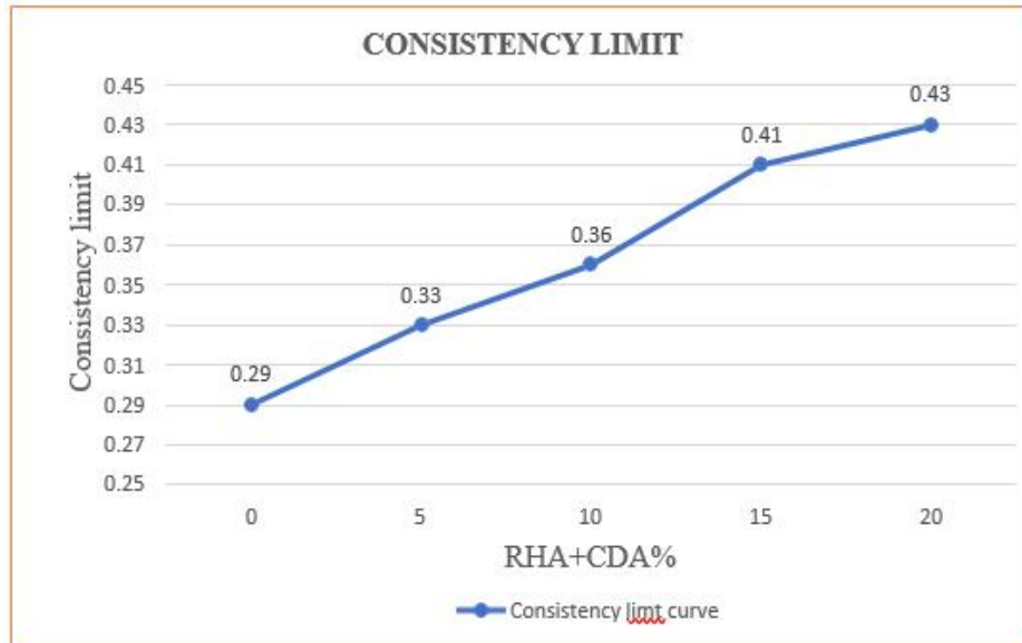
Fig. 3: Consistency curve for RHA+CDA concrete mix
