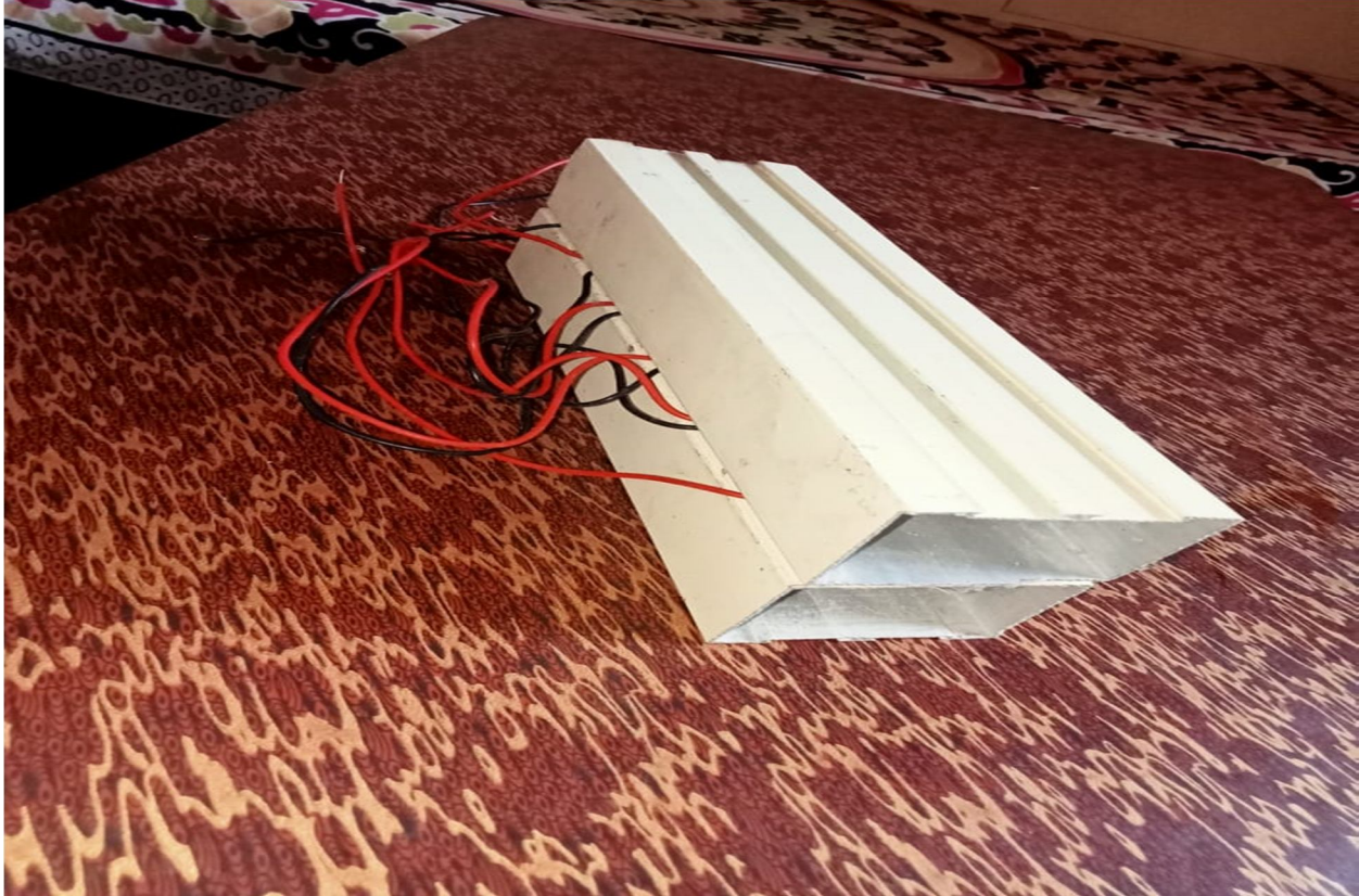
Figure 2. peltier sandwiched between hollow boxes
