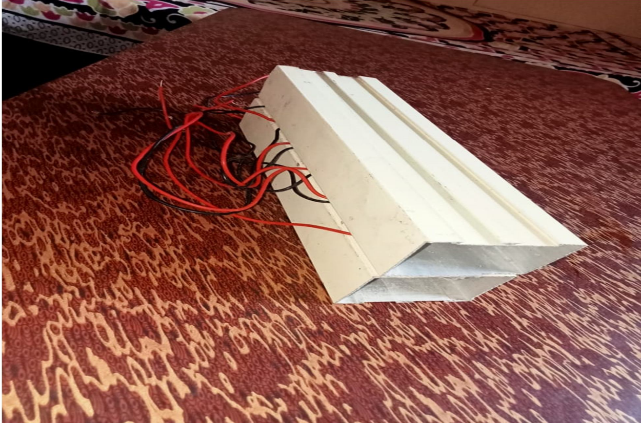
Figure 2. Peltier sandwiched between hollow boxes
