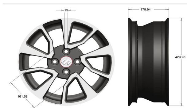
Fig. 3.2. Alloy wheel geometry
