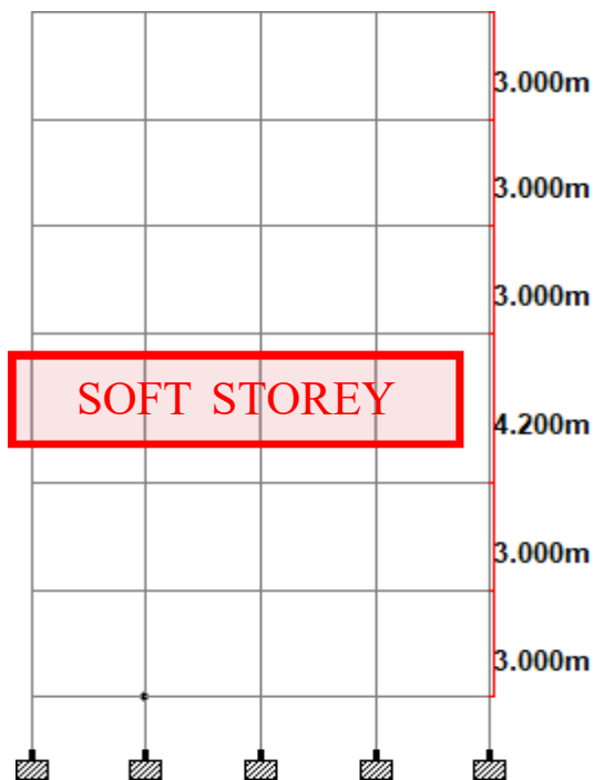
SOFT STOREY AT 2ND FLOOR
