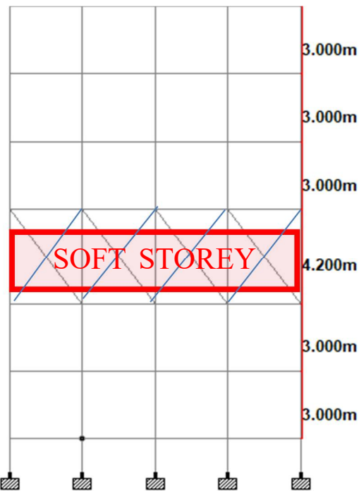
SECOND FLOOR SOFT STOREY WITH INCLINED COLUMN
