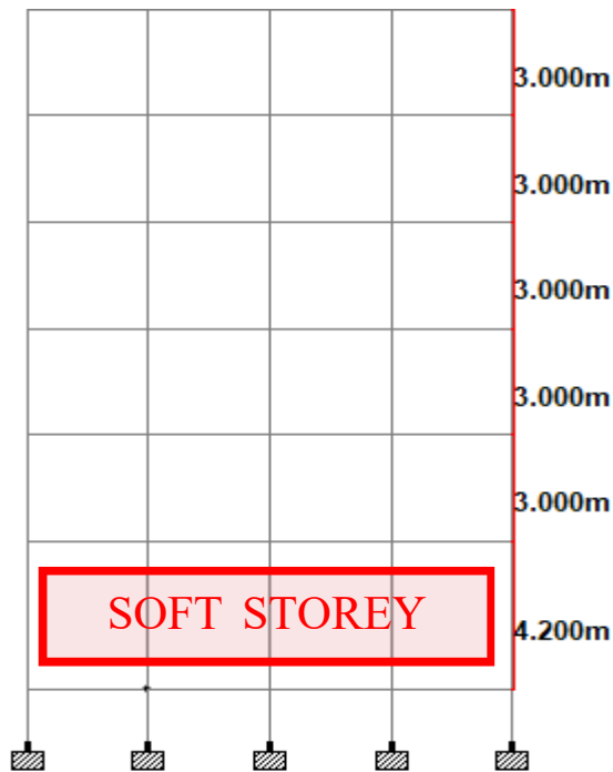
BARE FRAME SOFT STOREY AT GROUND
