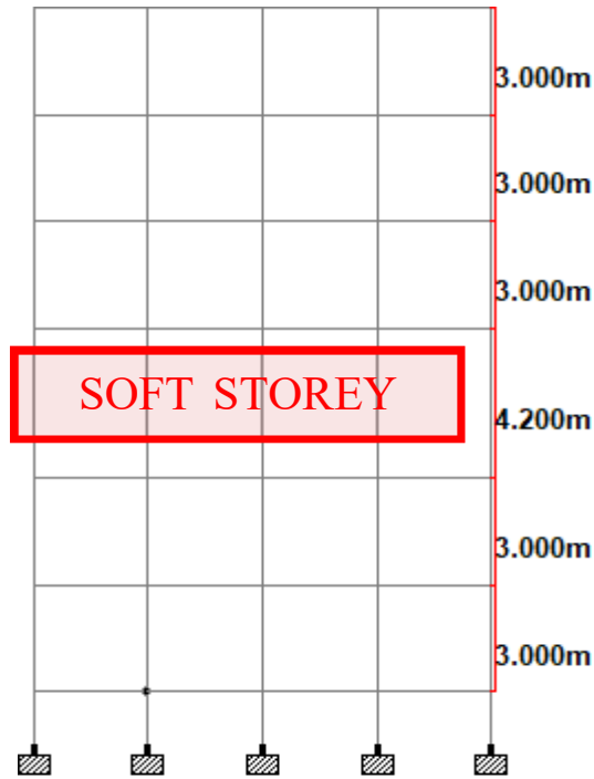
SOFT STOREY AT 2ND FLOOR
