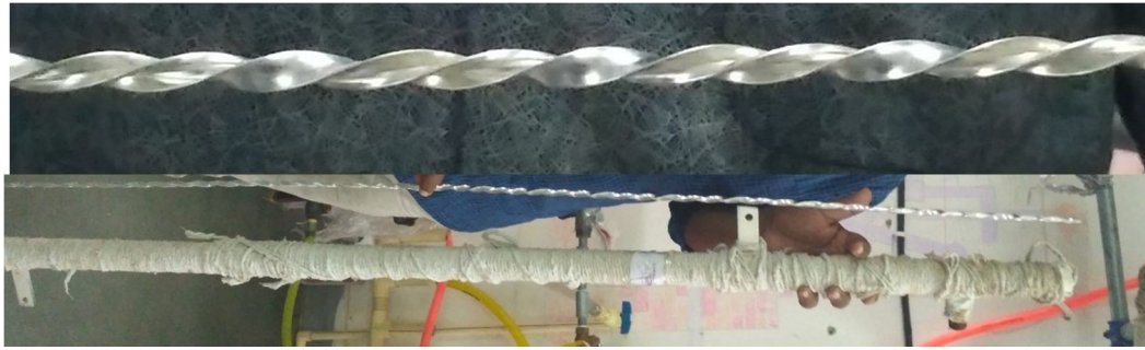
Fig. 2 Twisted tape insert and tube
