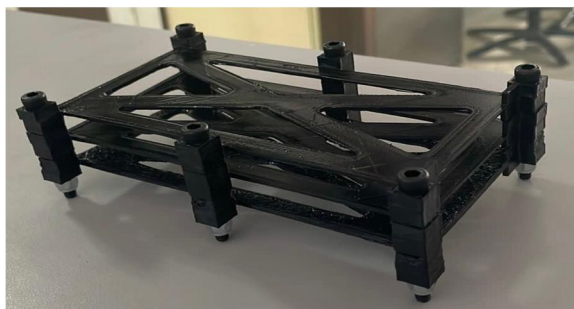
Fig. 8 Casing for pouch cell
