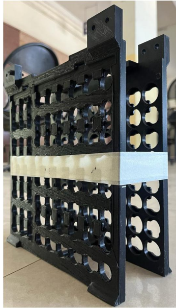
Fig. 9 Casing for Cylindrical Cell
