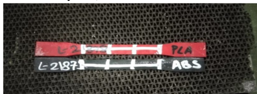
Fig. 5 Specimen post testing
