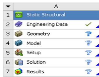
Fig-2: Static Structural Standalone System
