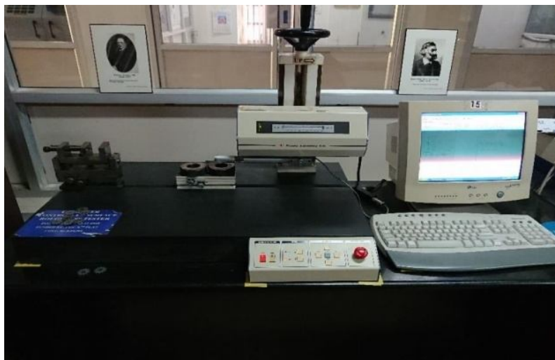
Figure 4.3 Computer controlled Surface Roughness Testing Machine
