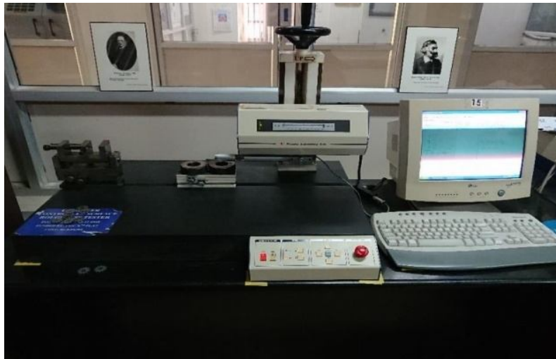
Figure 4.3 Computer controlled Surface Roughness Testing Machine
