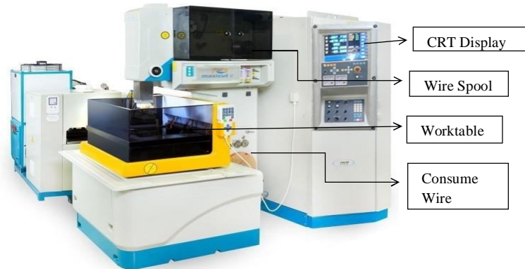
Figure 3.1 Pictorial view of MAXICUT CNC Wire EDM
