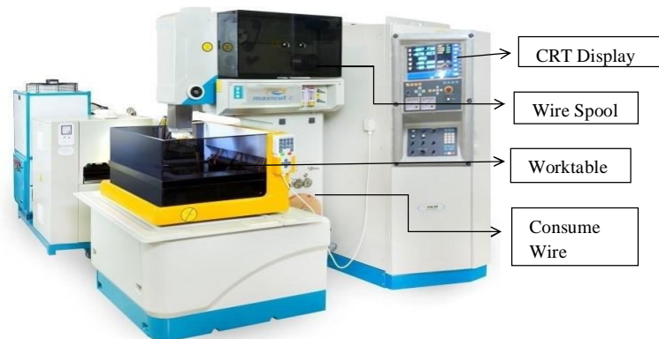
Figure 3.1 Pictorial view of MAXICUT CNC Wire EDM
