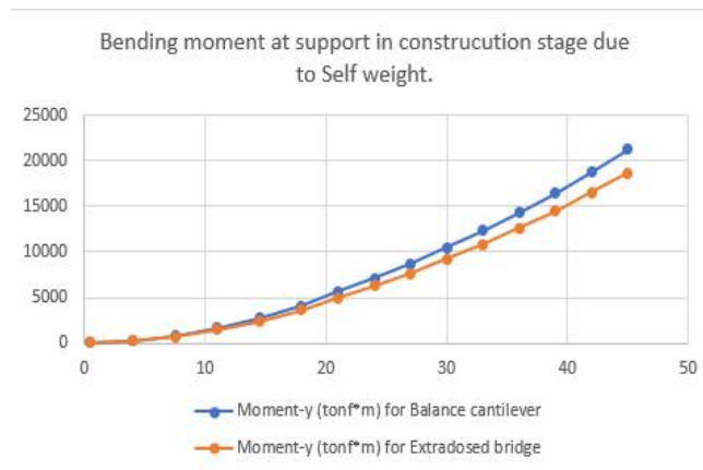
Fig. 10 Comparison of Bending moment at support in construction stage due to Dead Load
