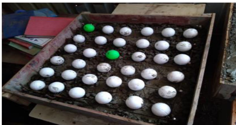
Fig-3: Location of plastic balls
