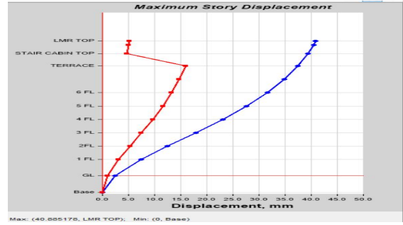
Story Displacement by Load Case SPEC X in Model 2
