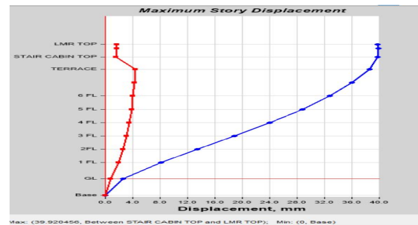
Story Displacement by Load Case EQX in Model 2
