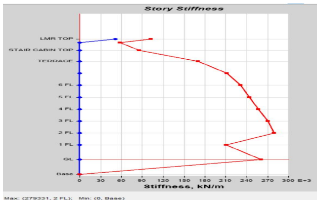
Story Stiffness by Load Case SPEC Y in Model 1
