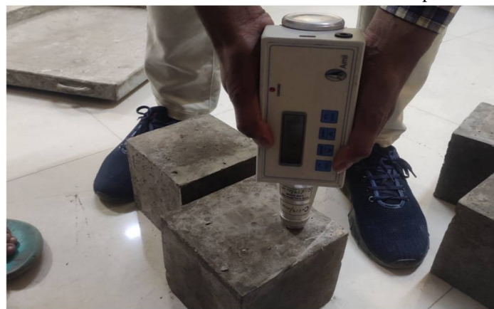
Figure- 4(Rebound Hammer Test)
