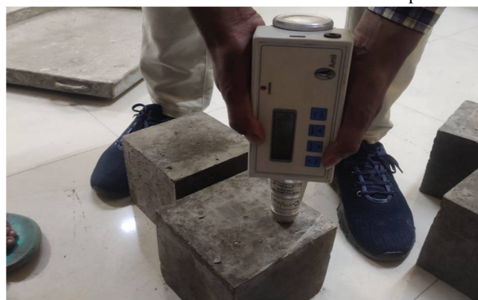
Figure- 4(Rebound Hammer Test)
