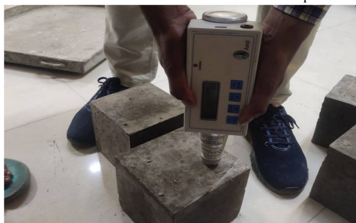
Figure- 4(Rebound Hammer Test)
