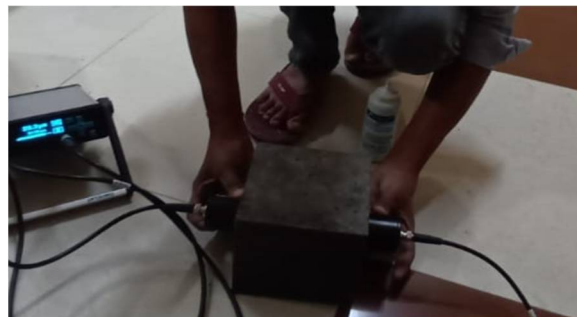
Figure- 6(Ultrasonic Pulse Velocity Test)
