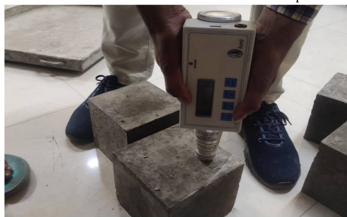
Figure- 4(Rebound Hammer Test)
