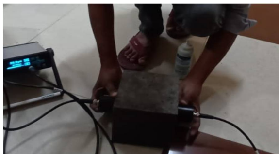
Figure- 6(Ultrasonic Pulse Velocity Test)
