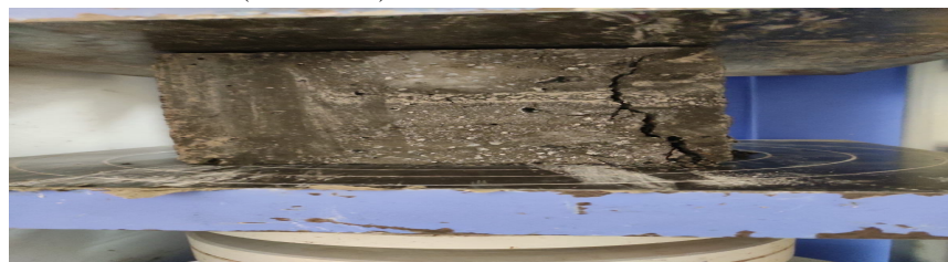
Fig. 3: Performing Compressive Strength Test
