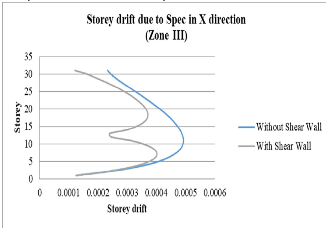
Graph 7 Storey Drift due to seismic load case Response Spectrum in X-direction for Zone III
