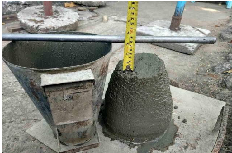
Fig. 2 Figure showing the slump test on fresh concrete
