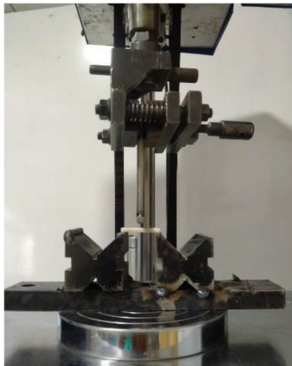
Figure 2. Experimental setup for flexural strength
