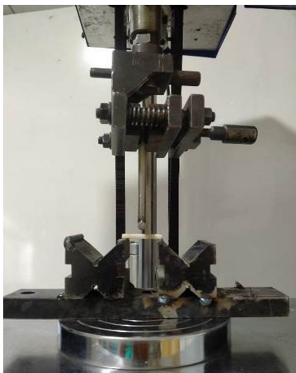
Figure 2. Experimental setup for flexural strength
