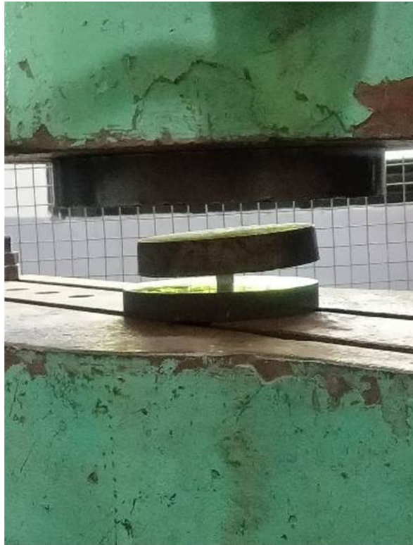
Figure 1. Experimental setup for Compression Test
