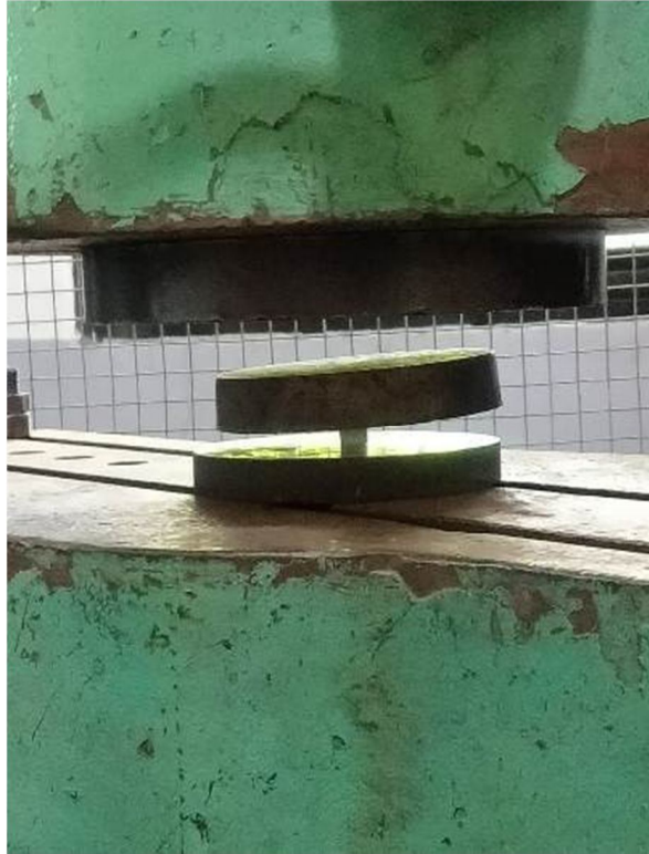
Figure 1. Experimental setup for Compression Test
