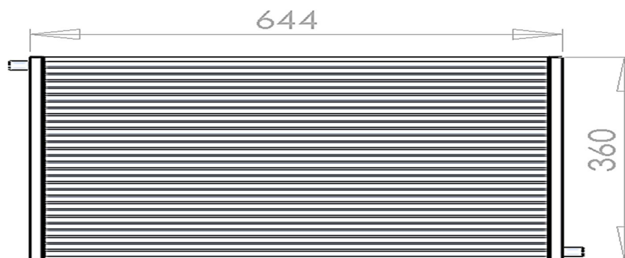
Figure 4.1 Radiator model in full dimensions (Solidworks)
