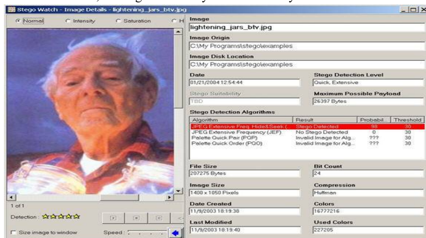
FIGURE 8: Information from Stego Watch about a JPEG file suspected to be a steganography carrier.
