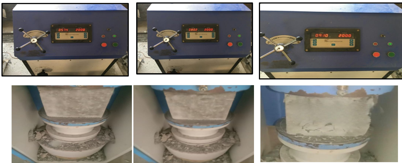
Figure 3: Testing Of Cubes On CTM
