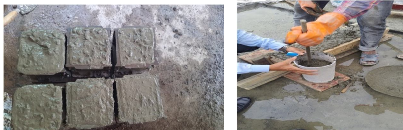
Figure 2: Casting of cubes, beam and cylinder
