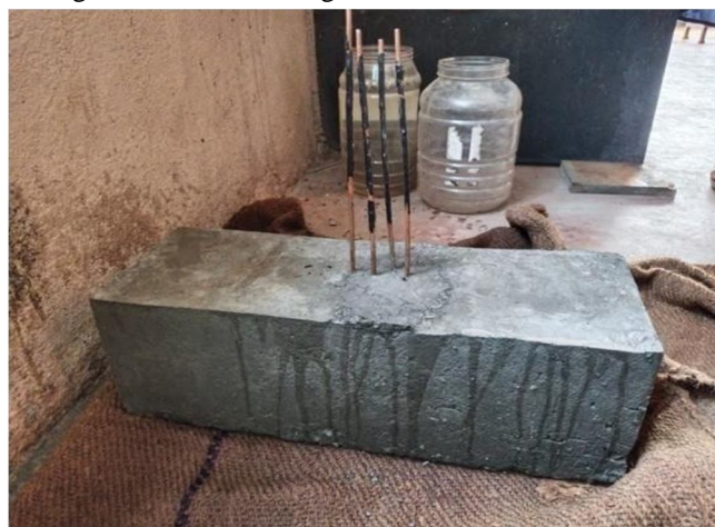
Fig.No.3.16) Curing of Beam
