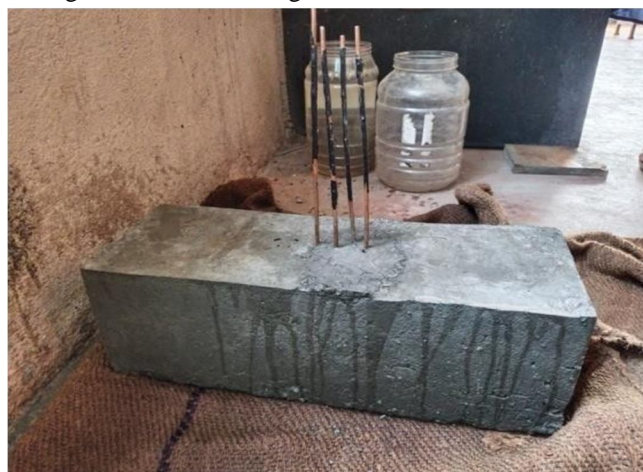
Fig.No.3.16) Curing of Beam
