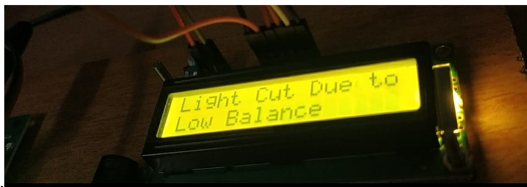
Fig 8: When energy meter cut off the load due to insufficient balance
