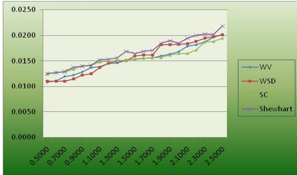
Fig 1.7 \bar{Z} and R charts type I risks of SC, W SD, W V and Shewhart charts for n = 7 of NovEPR distribution
