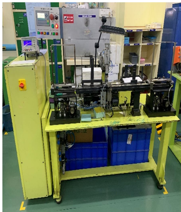
Fig 1.10 Coil unloading machine
