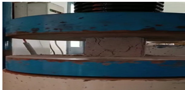
Fig.3 Figure showing AAC block under compression
