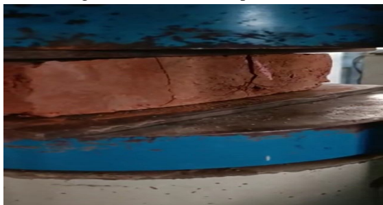
Fig.2 Figure showing Red clay brick under compression
