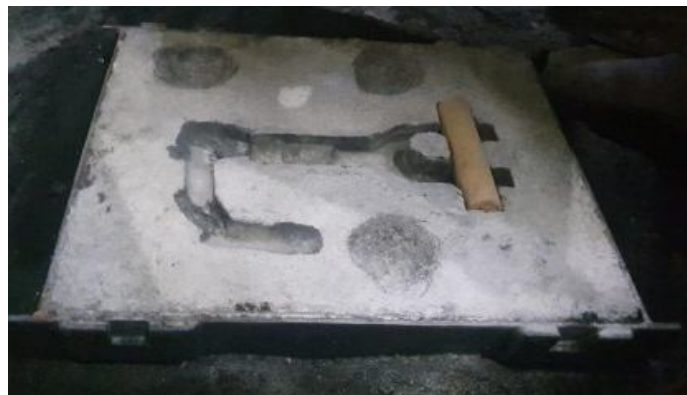
Fig. 3 Drag & Core placed horizontally
