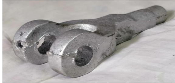
Fig. 13 Defective Fork End
