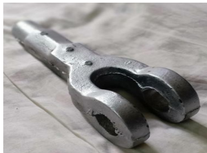
Fig. 12 Defect-free Fork End
