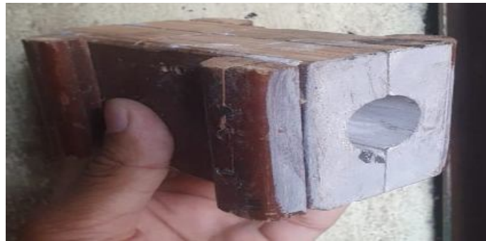
Fig. 2 Core box used for making core
