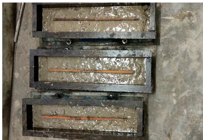
Photograph No. 2.1: casting of test specimen for accelerated corrosion test
