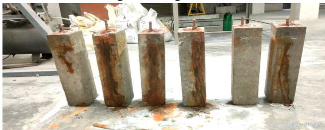
Photograph No. 4.4: Test specimen after accelerated corrosion test
