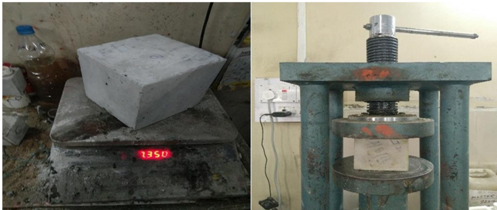
Fig. 1&2 Weight measurement and Compression testing machine
