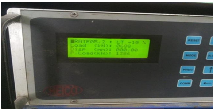
Fig. 3 Compressive load reading in KN
