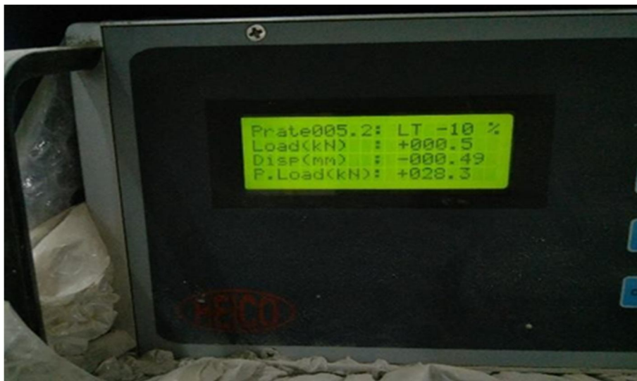
Fig. 6 Flexural load reading in KN
