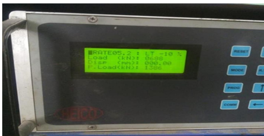
Fig. 3 Compressive load reading in KN
