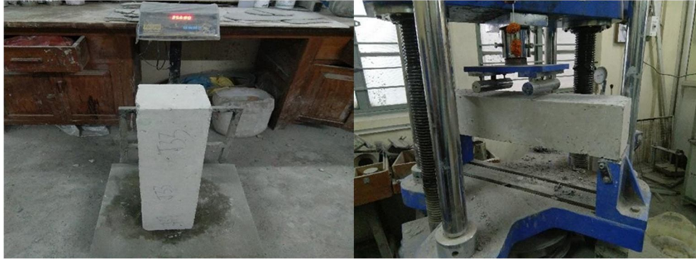
Fig. 4&5 Weight measurement and Flexural testing machine
