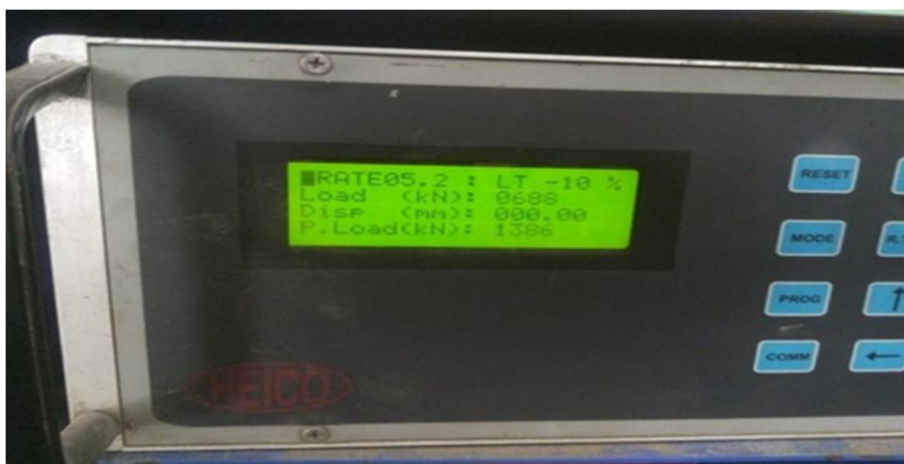
Fig. 3 Compressive load reading in KN
