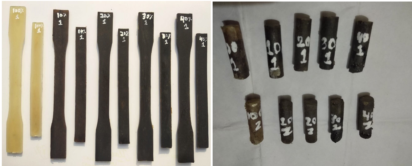
Fig 2 Tensile strength, flexural strength and wear test specimen of different composition
