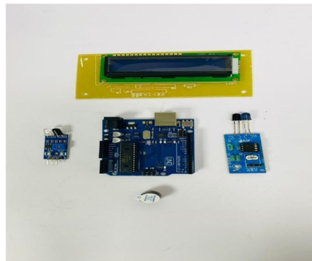
FIG 7. IR SENSORS, LCD DISPLAY, BUZZER, ARDUINO
