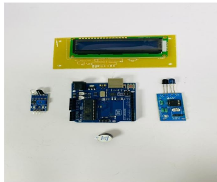
FIG 7. IR SENSORS, LCD DISPLAY, BUZZER, ARDUINO
