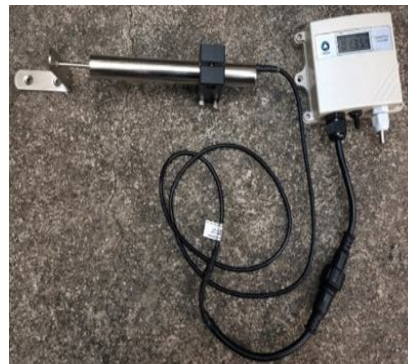
Fig.8: Installation of Linear variable displacement transformer instrument
