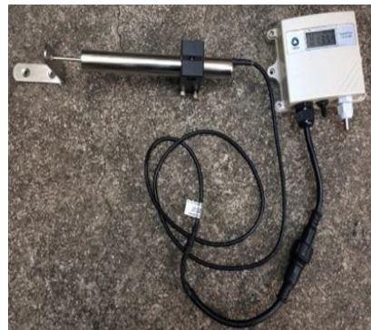
Fig.8: Installation of Linear variable displacement transformer instrument
