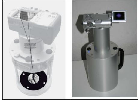
Fig 9 New digital crack monitoring device DRS
