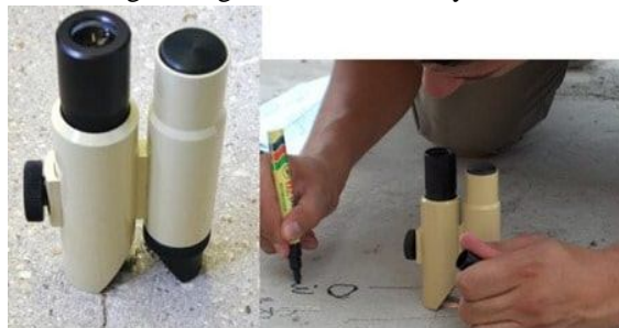
Fig.2: Crack Width Measurement Magnifier
