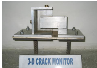
Fig 10 3-D crack monitor (3- dimensional crack monitor)
