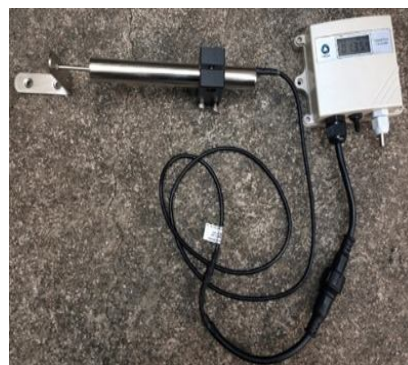
Fig.8: Installation of Linear variable displacement transformer instrument
