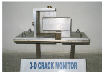
Fig 10 3-D crack monitor (3- dimensional crack monitor)
