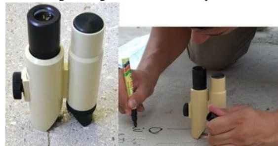
Fig.2: Crack Width Measurement Magnifier
