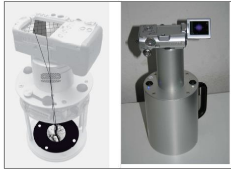
Fig 9 New digital crack monitoring device DRS
