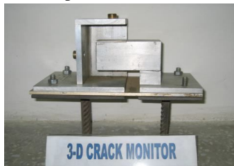
Fig 10 3-D crack monitor (3- dimensional crack monitor)
