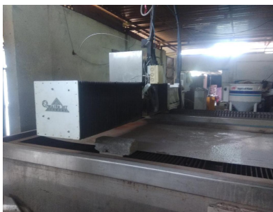
Fig: 1 Precision Abrasive Water Jet Machining Center manufactured by OMAX Corporation (Model: 2626)
