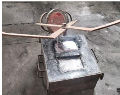
Fig 1: Pouring of molten aluminium
