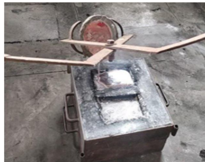
Fig 1: Pouring of molten aluminium
