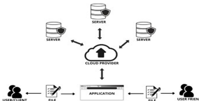
Fig. 1. Schema of centralized cloud-based storage system
