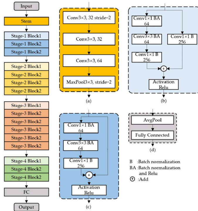
Fig. 1. Representation of XResNet Architecture
