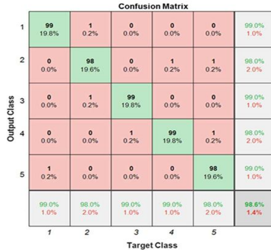
Fig. 7.4. Confusion matrix visualization for Corel dataset using InceptionResNetV2 architecture and CNN classifier
