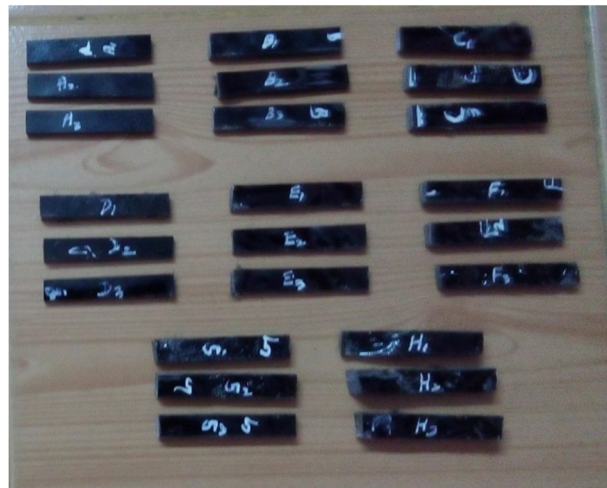
Figure 4.1 Specimens used for performing Impact test.
