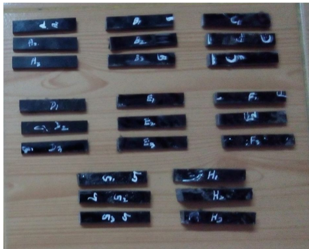
Figure 4.1 Specimens used for performing Impact test.
