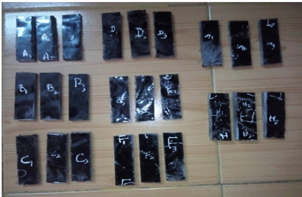
Figure 4.9 Specimens used for determining Density of Composites
