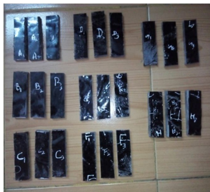
Figure 4.4 prepared Water Absorption test specimen
