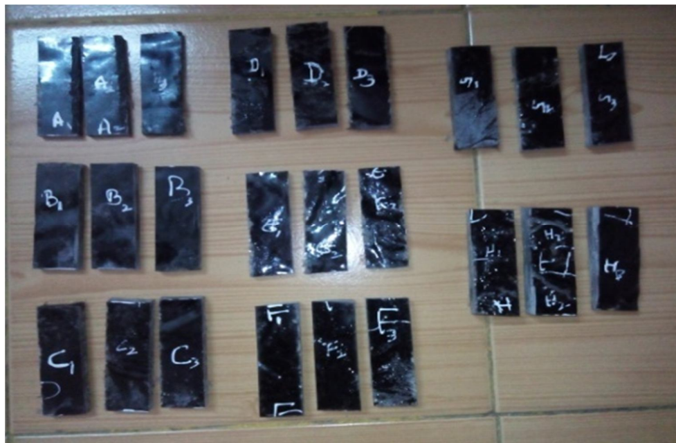
Figure 4.9 Specimens used for determining Density of Composites
