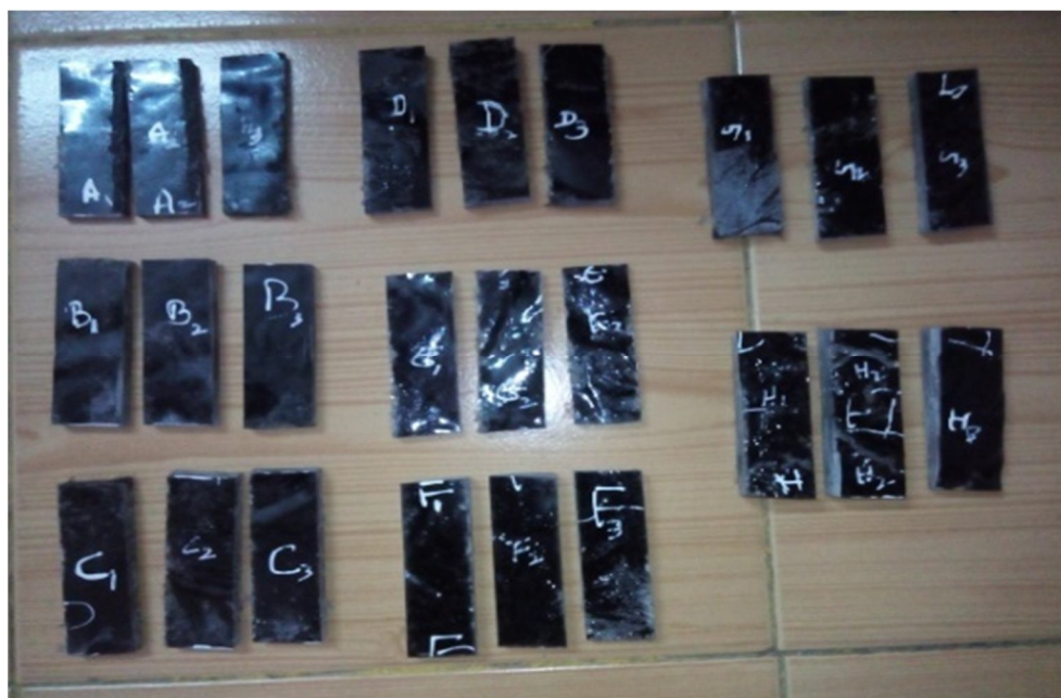
Figure 4.9 Specimens used for determining Density of Composites
