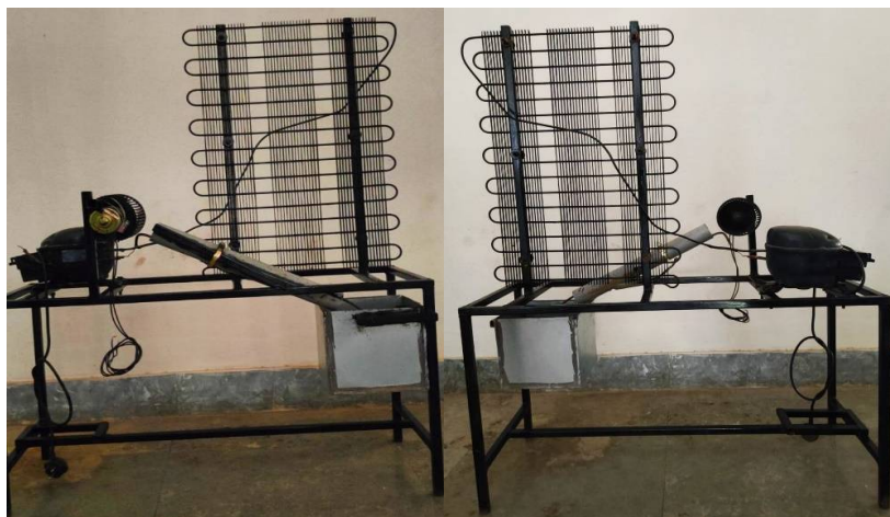
Fig. 4.2. Assembled Atmospheric Water Generator
