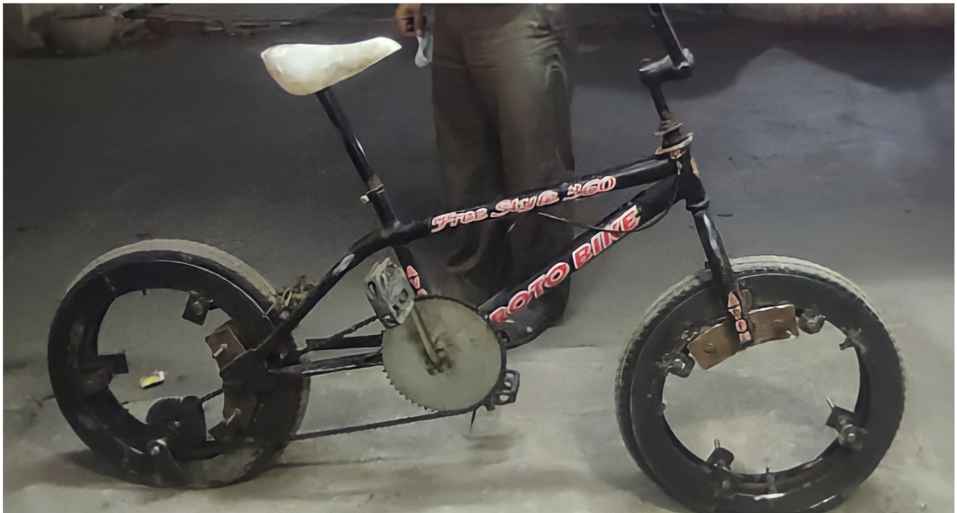
Fig.8: Assembly of Hubless Bicycle.
