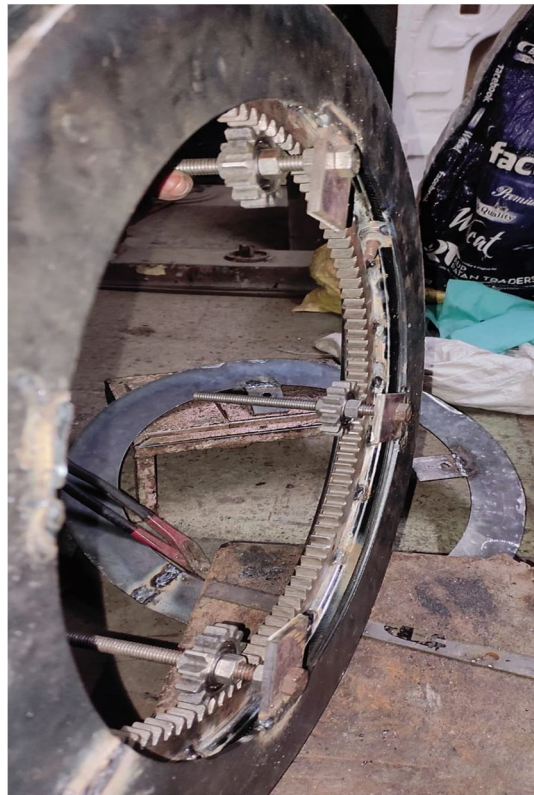
Fig.4: supporting spur gear.
