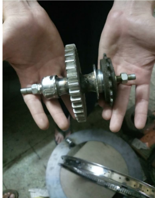
Fig.2: Spur Gear mounted on the hub.
