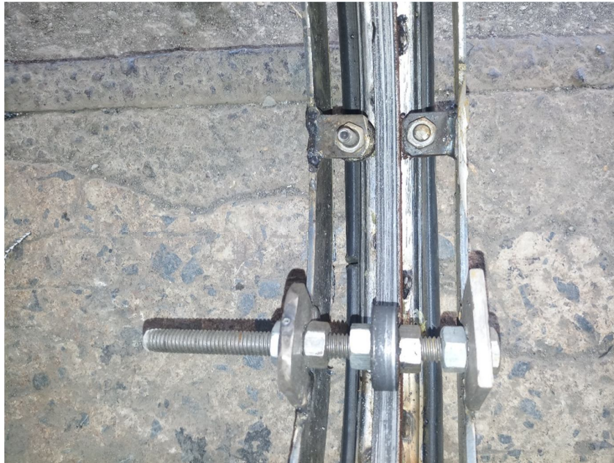
Fig.6: Support bearing mounted on M.S ring through nut and bolt and side bearing mounted on ring through nut and bolt.
